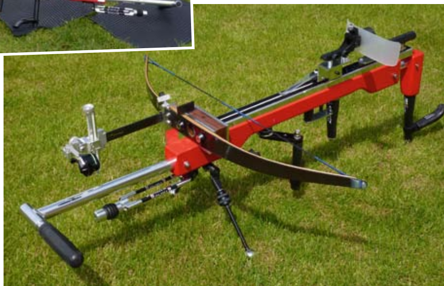
A machined aluminium track sits on top of the bow, preventing movement in the stock
